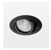
Recessed luminaire with LED, rated life of the LED L80/B10 50000 h (tambient 25°C), colour rendering index CRI > 96, chromaticity tolerance 2 SDCM (initial), reflector with circular light distribution pattern, reflector pure aluminium 99,99% in MIRO-Silver®, segmented and faceted, die-cast aluminium, powder-coated, rotation angle, swivel angle +/- 25°, black,
