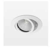
Recessed luminaire with LED, rated life of the LED L80/B10 50000 h (tambient 25°C), colour rendering index CRI > 96, chromaticity tolerance 2 SDCM (initial), reflector with circular light distribution pattern, reflector pure aluminium 99,99% in MIRO-Silver®, segmented and faceted, 3D lens silicon to reduce the proportion of scattered light, die-cast aluminium, powder-coated, rotation angle, swivel angle +/- 25°, white,
