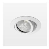
Recessed luminaire with LED, rated life of the LED L80/B10 50000 h (tambient 25°C), colour rendering index CRI > 80, chromaticity tolerance 2 SDCM (initial), reflector with circular light distribution pattern, reflector pure aluminium 99,99% in MIRO-Silver®, segmented and faceted, 3D lens silicon to reduce the proportion of scattered light, die-cast aluminium, powder-coated, rotation angle, swivel angle +/- 25°, white,
