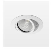
Recessed luminaire with LED, rated life of the LED L80/B10 50000 h (tambient 25°C), colour rendering index CRI > 90, chromaticity tolerance 2 SDCM (initial), reflector with circular light distribution pattern, reflector pure aluminium 99,99% in MIRO-Silver®, segmented and faceted, 3D lens silicon to reduce the proportion of scattered light, die-cast aluminium, powder-coated, rotation angle, swivel angle +/- 25°, white,
