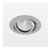
Recessed luminaire with LED, rated life of the LED L80/B10 50000 h (tambient 25°C), colour rendering index CRI > 96, chromaticity tolerance 2 SDCM (initial), reflector with circular light distribution pattern, reflector pure aluminium 99,99% in MIRO-Silver®, segmented and faceted, 3D lens silicon to reduce the proportion of scattered light, die-cast aluminium, powder-coated, rotation angle, swivel angle +/- 25°, silver,
