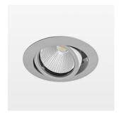
Recessed luminaire with LED, rated life of the LED L80/B10 50000 h (tambient 25°C), colour rendering index CRI > 80, chromaticity tolerance 2 SDCM (initial), reflector with circular light distribution pattern, reflector pure aluminium 99,99% in MIRO-Silver®, segmented and faceted, 3D lens silicon to reduce the proportion of scattered light, die-cast aluminium, powder-coated, rotation angle, swivel angle +/- 25°, silver,
