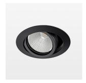
Recessed luminaire with LED, rated life of the LED L80/B10 50000 h (tambient 25°C), colour rendering index CRI > 96, chromaticity tolerance 2 SDCM (initial), reflector with circular light distribution pattern, reflector pure aluminium 99,99% in MIRO-Silver®, segmented and faceted, 3D lens silicon to reduce the proportion of scattered light, die-cast aluminium, powder-coated, rotation angle, swivel angle +/- 25°, black,
