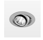
Recessed luminaire with LED, rated life of the LED L80/B10 50000 h (tambient 25°C), colour rendering index CRI > 80, chromaticity tolerance 2 SDCM (initial), rotation-symmetrical reflector with circular light distribution pattern, reflector pure aluminium 99,99% in MIRO-Silver®, segmented and faceted, 3D lens silicon to reduce the proportion of scattered light, die-cast aluminium, powder-coated, rotation angle, swivel angle +/- 25°, silver,
