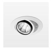
Recessed luminaire with LED, rated life of the LED L80/B10 50000 h (tambient 25°C), colour rendering index CRI > 96, chromaticity tolerance 2 SDCM (initial), rotation-symmetrical reflector with circular light distribution pattern, reflector pure aluminium 99,99% in MIRO-Silver®, segmented and faceted, 3D lens silicon to reduce the proportion of scattered light, die-cast aluminium, powder-coated, rotation angle, swivel angle +/- 25°, white,
