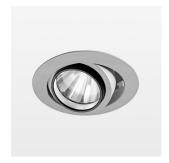
Recessed luminaire with LED, rated life of the LED L80/B10 50000 h (tambient 25°C), colour rendering index CRI > 90, chromaticity tolerance 2 SDCM (initial), rotation-symmetrical reflector with circular light distribution pattern, reflector pure aluminium 99,99% in MIRO-Silver®, segmented and faceted, 3D lens silicon to reduce the proportion of scattered light, die-cast aluminium, powder-coated, rotation angle, swivel angle +/- 25°, silver,
