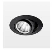
Recessed luminaire with LED, rated life of the LED L80/B10 50000 h (tambient 25°C), colour rendering index CRI > 96, chromaticity tolerance 2 SDCM (initial), rotation-symmetrical reflector with circular light distribution pattern, reflector pure aluminium 99,99% in MIRO-Silver®, segmented and faceted, 3D lens silicon to reduce the proportion of scattered light, die-cast aluminium, powder-coated, rotation angle, swivel angle +/- 25°, black,
