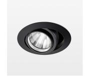
Recessed luminaire with LED, rated life of the LED L80/B10 50000 h (tambient 25°C), colour rendering index CRI > 90, chromaticity tolerance 2 SDCM (initial), rotation-symmetrical reflector with circular light distribution pattern, reflector pure aluminium 99,99% in MIRO-Silver®, segmented and faceted, 3D lens silicon to reduce the proportion of scattered light, die-cast aluminium, powder-coated, rotation angle, swivel angle +/- 25°, black,
