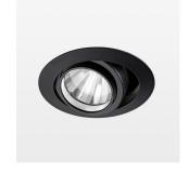
Recessed luminaire with LED, rated life of the LED L80/B10 50000 h (tambient 25°C), colour rendering index CRI > 80, chromaticity tolerance 2 SDCM (initial), rotation-symmetrical reflector with circular light distribution pattern, reflector pure aluminium 99,99% in MIRO-Silver®, segmented and faceted, 3D lens silicon to reduce the proportion of scattered light, die-cast aluminium, powder-coated, rotation angle, swivel angle +/- 25°, black,
