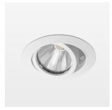
Recessed luminaire with LED, rated life of the LED L80/B10 50000 h (tambient 25°C), colour rendering index CRI > 90, chromaticity tolerance 2 SDCM (initial), rotation-symmetrical reflector with circular light distribution pattern, reflector pure aluminium 99,99% in MIRO-Silver®, segmented and faceted, 3D lens silicon to reduce the proportion of scattered light, die-cast aluminium, powder-coated, rotation angle, swivel angle +/- 25°, white,
