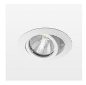
Recessed luminaire with LED, rated life of the LED L80/B10 50000 h (tambient 25°C), colour rendering index CRI > 80, chromaticity tolerance 3 SDCM (initial), rotation-symmetrical reflector with circular light distribution pattern, reflector pure aluminium 99,99% in MIRO-Silver®, segmented and faceted, 3D lens silicon to reduce the proportion of scattered light, die-cast aluminium, powder-coated, rotation angle, swivel angle +/- 25°, white,
