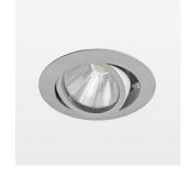
Recessed luminaire with LED, rated life of the LED L80/B10 50000 h (tambient 25°C), colour rendering index CRI > 90, chromaticity tolerance 2 SDCM (initial), rotation-symmetrical reflector with circular light distribution pattern, reflector pure aluminium 99,99% in MIRO-Silver®, segmented and faceted, 3D lens silicon to reduce the proportion of scattered light, die-cast aluminium, powder-coated, rotation angle, swivel angle +/- 25°, silver,
