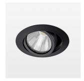
Recessed luminaire with LED, rated life of the LED L80/B10 50000 h (tambient 25°C), colour rendering index CRI > 95, chromaticity tolerance 2 SDCM (initial), rotation-symmetrical reflector with circular light distribution pattern, reflector pure aluminium 99,99% in MIRO-Silver®, segmented and faceted, 3D lens silicon to reduce the proportion of scattered light, die-cast aluminium, powder-coated, rotation angle, swivel angle +/- 25°, black,
