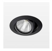
Recessed luminaire with LED, rated life of the LED L80/B10 50000 h (tambient 25°C), colour rendering index CRI > 90, chromaticity tolerance 3 SDCM (initial), rotation-symmetrical reflector with circular light distribution pattern, reflector pure aluminium 99,99% in MIRO-Silver®, segmented and faceted, 3D lens silicon to reduce the proportion of scattered light, die-cast aluminium, powder-coated, rotation angle, swivel angle +/- 25°, black,
