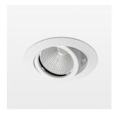
Recessed luminaire with LED, rated life of the LED L80/B10 50000 h (tambient 25°C), colour rendering index CRI > 80, chromaticity tolerance 2 SDCM (initial), reflector with circular light distribution pattern, reflector pure aluminium 99,99% in MIRO-Silver®, segmented and faceted, die-cast aluminium, powder-coated, rotation angle, swivel angle +/- 25°, white,
