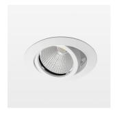
Recessed luminaire with LED, rated life of the LED L80/B10 50000 h (tambient 25°C), colour rendering index CRI > 90, chromaticity tolerance 2 SDCM (initial), reflector with circular light distribution pattern, reflector pure aluminium 99,99% in MIRO-Silver®, segmented and faceted, die-cast aluminium, powder-coated, rotation angle, swivel angle +/- 25°, white,
