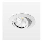
Recessed luminaire with LED, rated life of the LED L80/B10 50000 h (tambient 25°C), colour rendering index CRI > 80, chromaticity tolerance 2 SDCM (initial), reflector with oval light distribution pattern, reflector pure aluminium 99,99% in MIRO-Silver®, segmented, die-cast aluminium, powdercoated, rotation angle, swivel angle +/- 25°, white,
