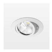
Recessed luminaire with LED, rated life of the LED L80/B10 50000 h (tambient 25°C), colour rendering index CRI > 90, chromaticity tolerance 2 SDCM (initial), reflector with oval light distribution pattern, reflector pure aluminium 99,99% in MIRO-Silver®, segmented, die-cast aluminium, powder-coated, rotation angle, swivel angle +/- 25°, white,
