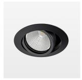
Recessed luminaire with LED, rated life of the LED L80/B10 50000 h (tambient 25°C), colour rendering index CRI > 90, chromaticity tolerance 2 SDCM (initial), reflector with circular light distribution pattern, reflector pure aluminium 99,99% in MIRO-Silver®, segmented and faceted, 3D lens silicon to reduce the proportion of scattered light, die-cast aluminium, powder-coated, rotation angle, swivel angle +/- 25°, black,
