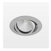
Recessed luminaire with LED, rated life of the LED L80/B10 50000 h (tambient 25°C), colour rendering index CRI > 96, chromaticity tolerance 2 SDCM (initial), reflector with circular light distribution pattern, reflector pure aluminium 99,99% in MIRO-Silver®, segmented and faceted, die-cast aluminium, powder-coated, rotation angle, swivel angle +/- 25°, silver,
