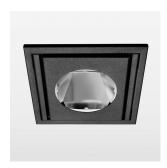
Recessed luminaire with LED, rated life of the LED L80/B10 > 50000 h, colour rendering index CRI > 90, chromaticity tolerance 2 SDCM (initial), reflector with circular light distribution pattern, reflector pure aluminium 99,99% in MIRO-Silver®,, swivel angle 30° luminaire housing sheet steel, powder-coated, black, separate driver unit
