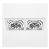
Recessed luminaire with LED, rated life of the LED L80/B10 > 50000 h, colour rendering index CRI > 90, chromaticity tolerance 2 SDCM (initial), reflector with circular light distribution pattern, swivel angle  $\pm$  30° luminaire housing sheet steel, powder-coated, white, separate driver unit
