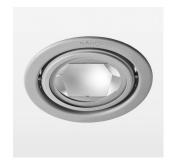
Recessed luminaire with LED, rated life of the LED L80/B10 > 50000 h, colour rendering index CRI > 70, chromaticity tolerance 2 SDCM (initial), reflector with circular light distribution pattern, reflector pure aluminium 99,99% in MIRO-Silver®, swivel angle +/-25°, luminaire housing sheet steel, powder-coated, silver, separate driver unit
