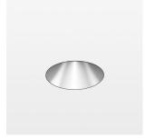
Recessed downlight, flush with ceiling with LED, rated life of the LED L80/B10 > 50000 h, colour rendering index CRI > 82, chromaticity tolerance 2 SDCM (initial), reflector with homogeneous light distribution pattern, diffuser lens, translucent, darklight reflector, aluminium, metallised, highgloss, luminaire head die-cast aluminium,
