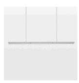
Suspended luminaire with LED, rated life of the LED L90/B50 50000 h (tambient 25°C), colour rendering index CRI > 80, chromaticity tolerance 3 SDCM (initial), extra wide, homogeneous light distribution pattern (90°), TIR-lens made of PMMA, luminaire housing sheet steel, powder-coated, matt silver, power supply via suspension cables
