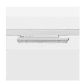
Surface-mounted luminaire with LED, rated life of the LED L90/B50 50000 h (tambient 25°C), colour rendering index CRI > 80, chromaticity tolerance 3 SDCM (initial), extra wide, homogeneous light distribution pattern (90°), TIR-lens made of PMMA, luminaire housing sheet steel, powder-coated, white, locking mechanism to aligned in 15° steps, rotation angle 300°, In-Track-Adapter, Casambi, On/Off, 220-240 V~ / 50-60 Hz, max. 64 luminaires per circuit (B16A fuse)
