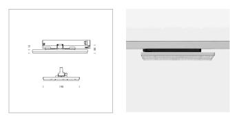
Surface-mounted luminaire with LED, rated life of the LED L90/B50 50000 h (tambient 25°C), colour rendering index CRI > 80, chromaticity tolerance 3 SDCM (initial), extra wide, homogeneous light distribution pattern (90°), TIR-lens made of PMMA, luminaire housing sheet steel, powder-coated, silver, locking mechanism to aligned in 15° steps, rotation angle 300°, In-Track-Adapter, Casambi, 220-240 V~ / 50-60 Hz, max. 64 luminaires per circuit (B16A fuse)
