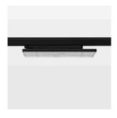
Surface-mounted luminaire with LED, rated life of the LED L90/B50 50000 h (tambient 25°C), colour rendering index CRI > 80, chromaticity tolerance 3 SDCM (initial), extra wide, homogeneous light distribution pattern (90°), TIR-lens made of PMMA, luminaire housing sheet steel, powder-coated, black, locking mechanism to aligned in 15° steps, rotation angle 300°, In-Track-Adapter, Casambi, 220-240 V~ / 50-60 Hz, max. 64 luminaires per circuit (B16A fuse)
