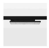
Surface-mounted luminaire with LED, rated life of the LED L90/B50 50000 h (tambient 25°C), colour rendering index CRI > 80, chromaticity tolerance 3 SDCM (initial), wide, homogeneous light distribution pattern (60°), TIR-lens made of PMMA, luminaire housing sheet steel, powder-coated, black, locking mechanism to aligned in 15° steps, rotation angle 300°, In-Track-Adapter, Casambi, 220-240 V~/50-60 Hz, max. 64 luminaires per circuit (B16A fuse)
