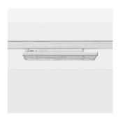
Surface-mounted luminaire with LED, rated life of the LED L90/B50 50000 h (tambient 25°C), colour rendering index CRI > 80, chromaticity tolerance 3 SDCM (initial), wide, homogeneous light distribution pattern 30°, TIR-lens made of PMMA, luminaire housing sheet steel, powder-coated, white, locking mechanism to aligned in 15° steps, rotation angle 300°, In-Track-Adapter, Casambi, On/Off, 220-240 V~ / 50-60 Hz, max. 64 luminaires per circuit (B16A fuse)
