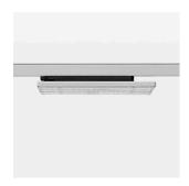
Surface-mounted luminaire with LED, rated life of the LED L90/B50 50000 h (tambient 25°C), colour rendering index CRI > 80, chromaticity tolerance 3 SDCM (initial), wide, homogeneous light distribution pattern 30°, TIR-lens made of PMMA, luminaire housing sheet steel, powder-coated, silver, locking mechanism to aligned in 15° steps, rotation angle 300°, In-Track-Adapter, Casambi, 220-240 V~/50-60 Hz, max. 64 luminaires per circuit (B16A fuse)
