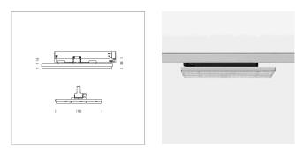
Surface-mounted luminaire with LED, rated life of the LED L90/B50 50000 h (tambient 25°C), colour rendering index CRI > 80, chromaticity tolerance 3 SDCM (initial), wide, homogeneous light distribution pattern (60°), TIR-lens made of PMMA, luminaire housing sheet steel, powder-coated, silver, locking mechanism to aligned in 15° steps, rotation angle 300°, In-Track-Adapter, On/Off, 220-240 V~ / 50-60 Hz, max. 27 luminaires per circuit (B16A fuse)
