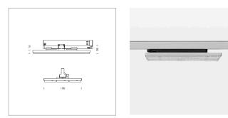
Surface-mounted luminaire with LED, rated life of the LED L90/B50 50000 h (tambient 25°C), colour rendering index CRI > 80, chromaticity tolerance 3 SDCM (initial), wide, homogeneous light distribution pattern 30°, TIR-lens made of PMMA, luminaire housing sheet steel, powder-coated, silver, locking mechanism to aligned in 15° steps, rotation angle 300°, In-Track-Adapter, On/Off, 220-240 V~ / 50-60 Hz, max. 27 luminaires per circuit (B16A fuse)
