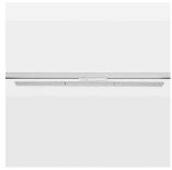
Surface-mounted luminaire with LED, rated life of the LED L90/B50 50000 h (tambient 25°C), colour rendering index CRI > 80, chromaticity tolerance 3 SDCM (initial), extra wide, homogeneous light distribution pattern (90°), TIR-lens made of PMMA, luminaire housing sheet steel, powder-coated, white, locking mechanism to aligned in 15° steps, rotation angle 300°, In-Track-Adapter, On/Off, 220-240 V~ / 50-60 Hz
