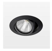
Recessed luminaire with LED, rated life of the LED L80/B10 50000 h (tambient 25°C), colour rendering index CRI > 80, chromaticity tolerance 3 SDCM (initial), rotation-symmetrical reflector with circular light distribution pattern, reflector pure aluminium 99,99% in MIRO-Silver®, segmented and faceted, 3D lens silicon to reduce the proportion of scattered light, die-cast aluminium, powder-coated, rotation angle, swivel angle +/- 25°, black,
