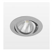
Recessed luminaire with LED, rated life of the LED L80/B10 50000 h (tambient 25°C), colour rendering index CRI > 80, chromaticity tolerance 3 SDCM (initial), rotation-symmetrical reflector with circular light distribution pattern, reflector pure aluminium 99,99% in MIRO-Silver®, segmented and faceted, 3D lens silicon to reduce the proportion of scattered light, die-cast aluminium, powder-coated, rotation angle, swivel angle +/- 25°, silver,
