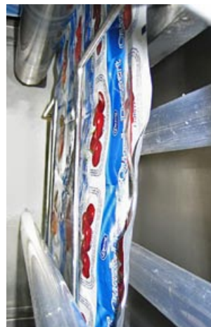
UV-C disinfection of foil covers
