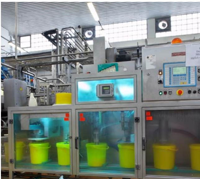
UV-C disinfection in the yoghurt filling area
