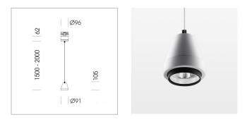
Suspended luminaire with LED, rated life of the LED L80/B10 > 50000 h, colour rendering index CRI > 96, chromaticity tolerance 2 SDCM (initial), reflector with circular light distribution pattern, reflector pure aluminium 99,99% in MIRO-Silver®,segmented and faceted, 3D lens silicon to reduce the proportion of scattered light, luminaire head die-cast aluminium, powder-coated, white
