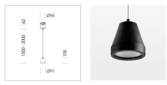
Suspended luminaire with LED, rated life of the LED L80/B10 > 50000 h, colour rendering index CRI > 90, chromaticity tolerance 2 SDCM (initial), reflector with circular light distribution pattern, reflector pure aluminium 99,99% in MIRO-Silver®,segmented and faceted, luminaire head die-cast aluminium, powder-coated, black
