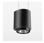
Suspended luminaire with LED, rated life of the LED L80/B10 50000 h (tambient 25°C), colour rendering index CRI > 70, chromaticity tolerance 2 SDCM (initial), reflector with circular light distribution pattern, 3D silicone lens to reduce the proportion of scattered light, reflector pure aluminium 99,99% in MIRO-Silver®, segmented and faceted, exchangeable reflector unit in high-sheen black plastic, with glass cover, luminaire housing die-cast aluminium, powder-coated, black
