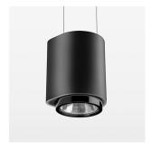
Suspended luminaire with LED, rated life of the LED L80/B10 50000 h (tambient 25°C), colour rendering index CRI > 80, chromaticity tolerance 2 SDCM (initial), reflector with circular light distribution pattern, 3D silicone lens to reduce the proportion of scattered light, reflector pure aluminium 99,99% in MIRO-Silver®, segmented and faceted, exchangeable reflector unit in high-sheen black plastic, with glass cover, luminaire housing die-cast aluminium, powder-coated, black
