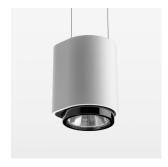
Suspended luminaire with LED, rated life of the LED L80/B10 50000 h (tambient 25°C), colour rendering index CRI > 82, chromaticity tolerance 2 SDCM (initial), reflector with oval light distribution pattern, 3D silicone lens to reduce the proportion of scattered light, reflector pure aluminium 99,99% in MIRO-Silver®, segmented, exchangeable reflector unit in high-sheen black plastic, with glass cover, luminaire housing die-cast aluminium, powdercoated, white
