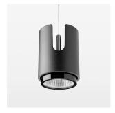
Suspended luminaire with LED, rated life of the LED L80/B10 50000 h (tambient 25°C), colour rendering index CRI > 96, chromaticity tolerance 3 SDCM (initial), reflector with circular light distribution pattern, reflector pure aluminium 99,99% in MIRO-Silver®, segmented and faceted, exchangeable reflector unit in high-sheen black plastic, with glass cover, luminaire housing die-cast aluminium, powder-coated, black
