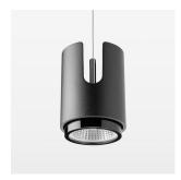
Suspended luminaire with LED, rated life of the LED L80/B10 50000 h (tambient 25°C), colour rendering index CRI > 96, chromaticity tolerance 2 SDCM (initial), reflector with circular light distribution pattern, 3D silicone lens to reduce the proportion of scattered light, reflector pure aluminium 99,99% in MIRO-Silver®, segmented and faceted, exchangeable reflector unit in high-sheen black plastic, with glass cover, luminaire housing die-cast aluminium, powder-coated, black
