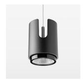
Suspended luminaire with LED, rated life of the LED L80/B10 50000 h (tambient 25°C), colour rendering index CRI > 96, chromaticity tolerance 2 SDCM (initial), reflector with circular light distribution pattern, reflector pure aluminium 99,99% in MIRO-Silver®, segmented and faceted, exchangeable reflector unit in high-sheen black plastic, with glass cover, luminaire housing die-cast aluminium, powder-coated, black
