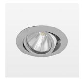
Recessed luminaire with LED, rated life of the LED L80/B10 50000 h (tambient 25°C), colour rendering index CRI > 90, chromaticity tolerance 3 SDCM (initial), rotation-symmetrical reflector with circular light distribution pattern, reflector pure aluminium 99,99% in MIRO-Silver®, segmented and faceted, 3D lens silicon to reduce the proportion of scattered light, die-cast aluminium, powder-coated, rotation angle, swivel angle +/- 25°, silver,
